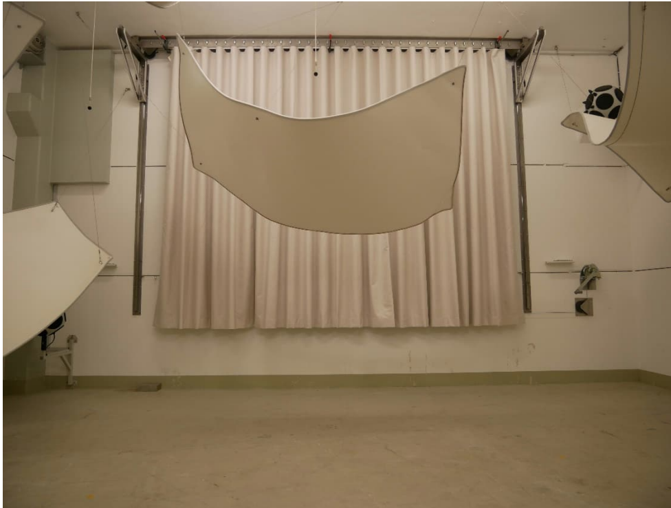
Figure B.1. Folded hanging curtain in the reverberation room: frontal view.
