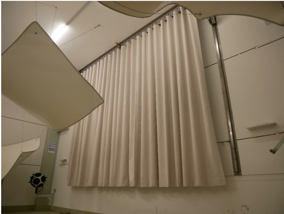
Figure B.2. Folded hanging curtain in the reverberation room: diagonal view.
